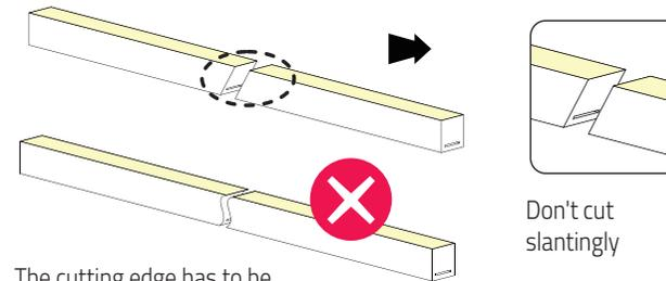
The cutting edge has to be smooth and needs to be sliced in angle of 90°.
