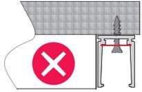
Screw head above to the base of aluminum profile.
