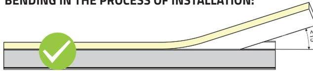
Installing angle should be less than 15 degree when pressing the light to the aluminum profile by hand.
