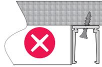
Gradient installing of screw.
