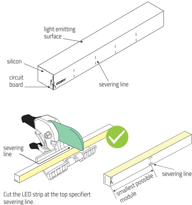
Place the LED strip and cut to the circuit board in a lying shape.
