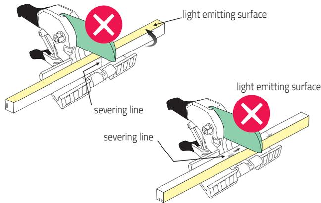
Cut the LED strip exactly at the specified severing lines - never between the marks.
