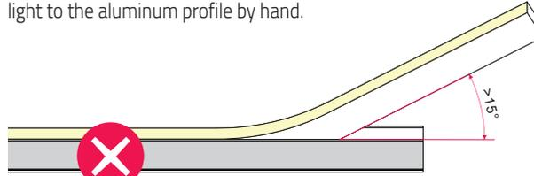
The circuit board could be damaged if installing angle larger than 15 degree.
