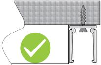
Install the screw into position and ensure the screw head is flush or lower the base of aluminum profile.
